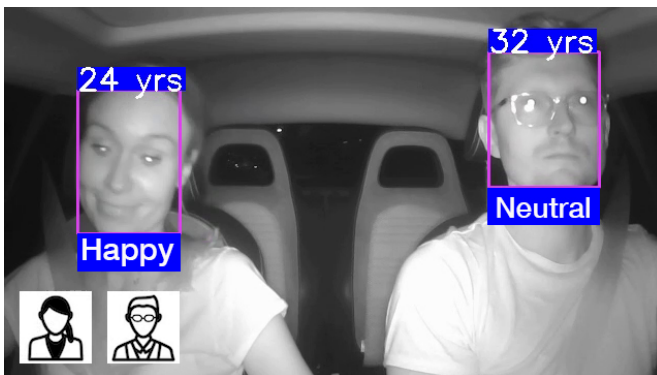
Figure 1. Our emotion recognition model in passenger detection system for autonomous cars. Emotion recognition is performed on detected facial regions
